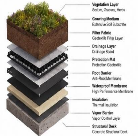
Green Roof System Detail
